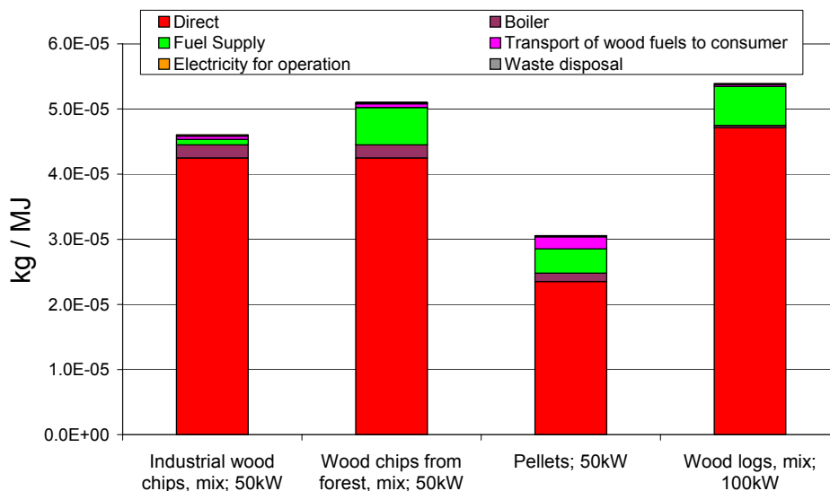
Fig. 9.2 Particle emissions <2.5 µm from different wood heating systems of the 50/100 kW class [kg/MJ useful energy].
